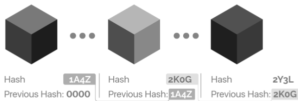
Figure 2: A chain of blocks that refers to the previous block in each node.
